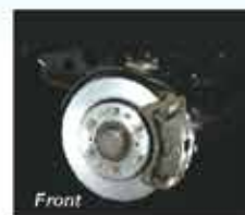
15-inch Ventilated Disc Brakes
